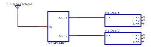
This application shows a single receive antenna split to two intercom base-stations.
