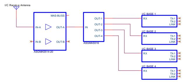
This application shows a single receive antenna split to four intercom base-stations with a RF Preamplifier included to overcome losses.
