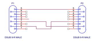
Wire can be shielded two-conductor or unshielded with a minimum of three conductors. Standard microphone cable is well suited.
